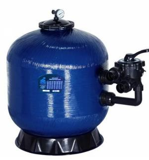
injection molded PVC. UV-resistance surface allows working under sunshine. Easy-to-use six-position valve makes you select any of the valve/filter operation in a proper way.
